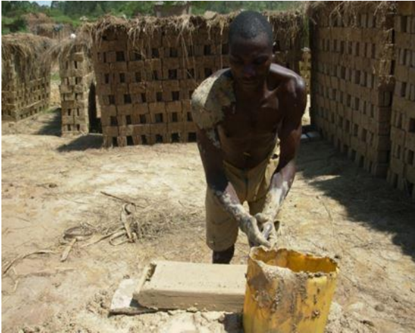
Figure 7. Brick making using a wooden mould.
