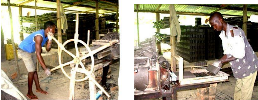
Figure 13. Production of face bricks using a manual operated extruder.
