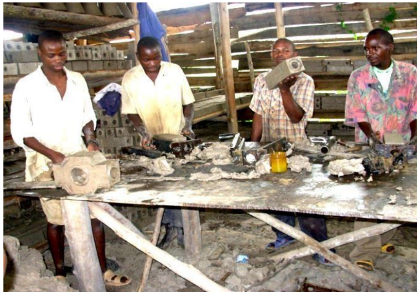
Figure 14. Forming process of bottom brick plates.
