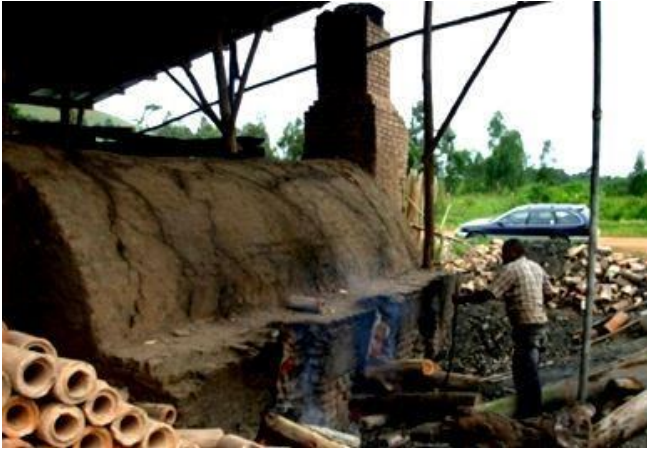
Figure 17. Firing bottom brick plates in a built kiln.
