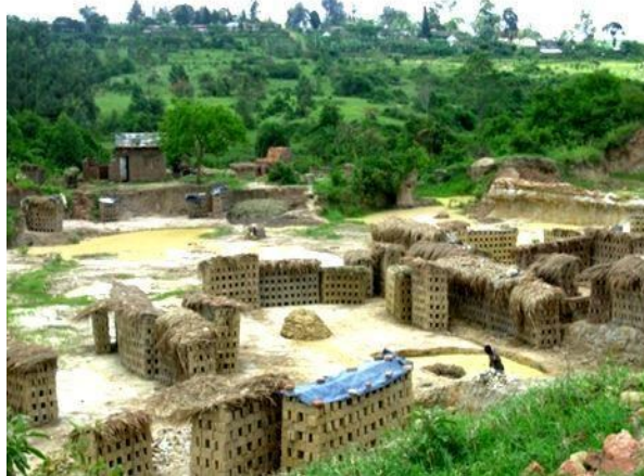
Figure 8. Stack bricks covered with grass.
