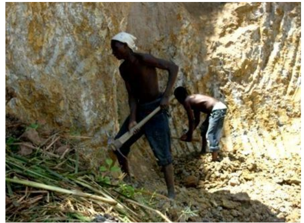
Figure 5. Extracting clay at a quarry for brick making.
