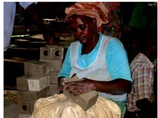
Figure 16. Trimming bottom brick plates.
