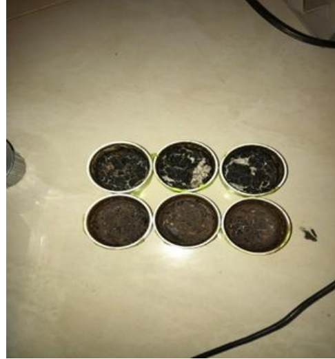
Figure 24 fecal sludge samples in the weighing balance and after they have been oven-dried.
