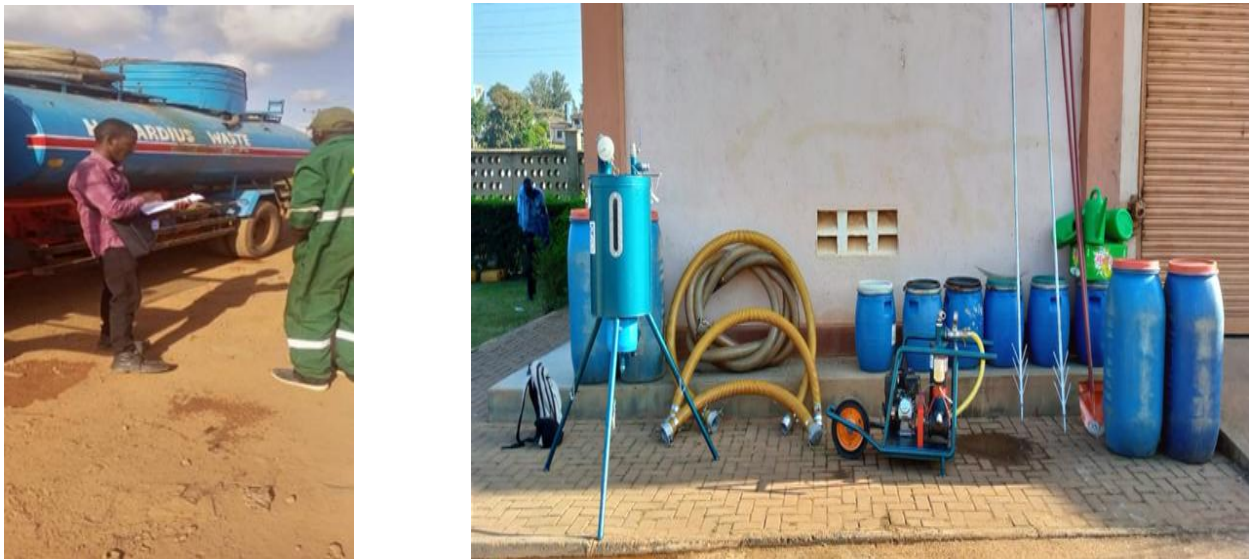
Figure 6 Administering questionnaires to onsite emptying technology operators and equipment used in the emptying process.
