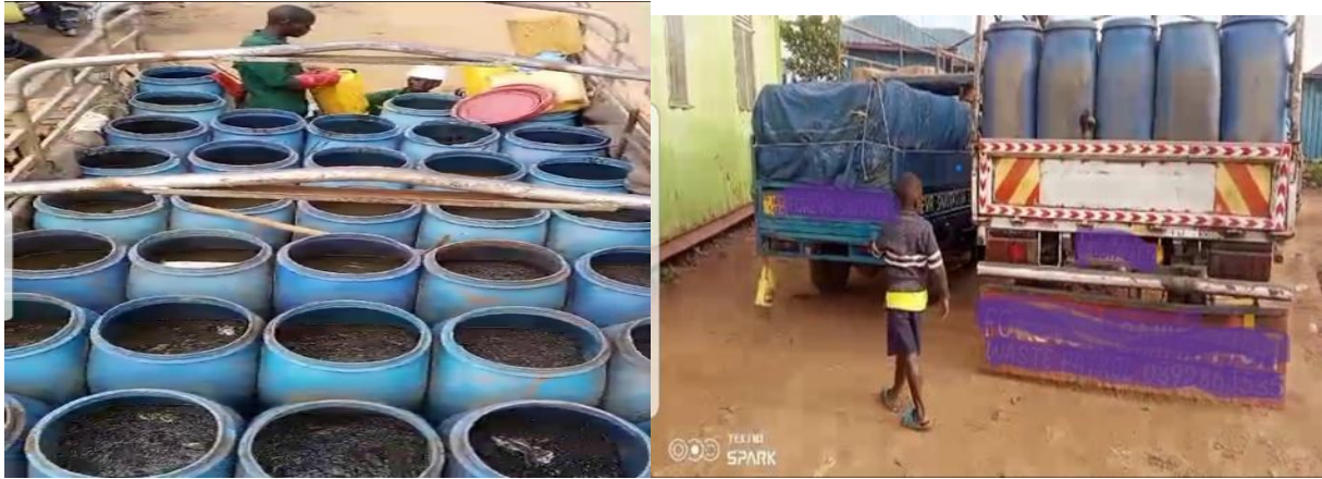
Figure 13 Drums with FS loaded on a truck and a tricycle for transportation to the Lubigi FSTP.
