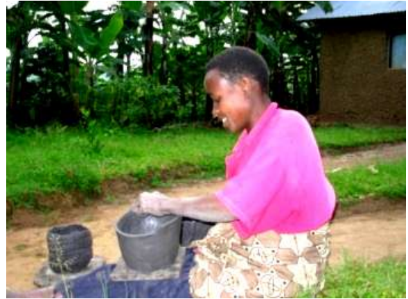
Figure 3. Making clay stoves using coils.
