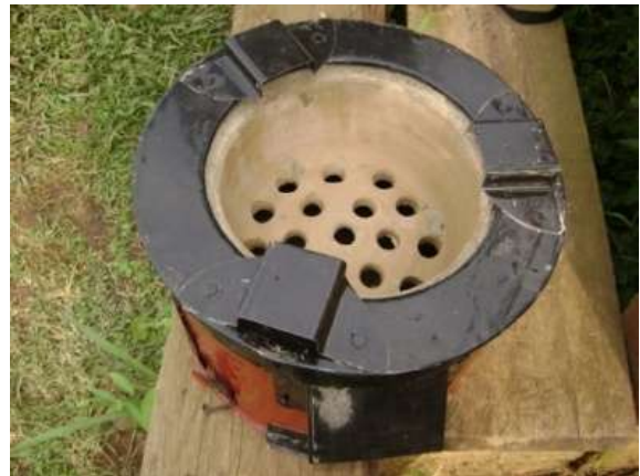
Figure 15. Energy saving stove with a ceramic insert.
