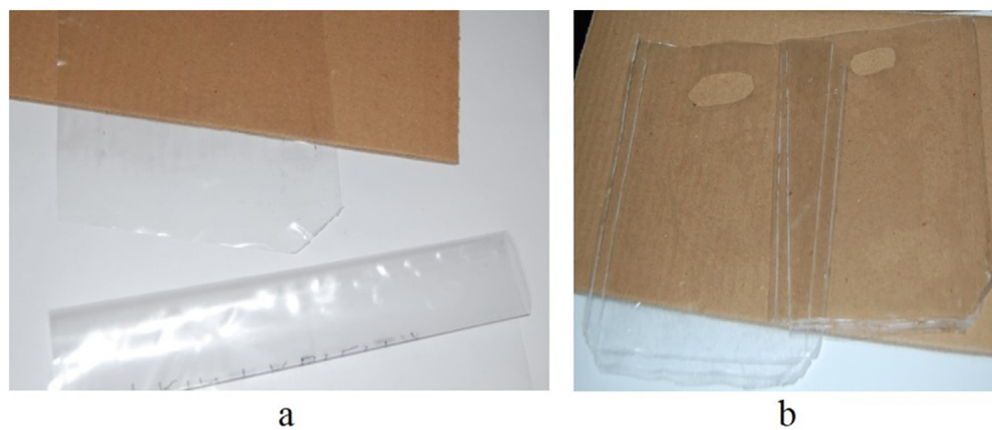
Fig. 7 – Film prototypes dried using a rangehood, as a roll (a) and bag (b).
